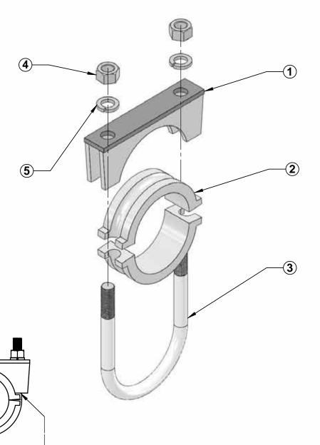
NOTE: - Insure equal amount of space on each side before tightening U-Bolts . - Insure equal number of threads on each side of U-Bolt.
